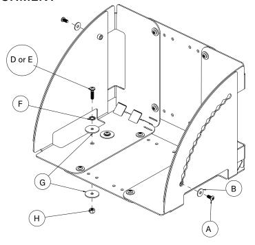
**FIGURE 3: ANGLE ADJUSTMENT**
